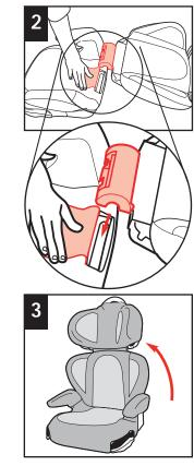
Insert the hook on the backrest into the large opening on back of seat base. Make sure backrest is laying flat (horizontal) when connecting. Make sure seat pad does not get caught between the moving parts.
